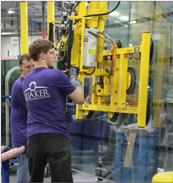
QUAKER USES glass manipulators (left) to move large glass units in the manufacturing facility. Chief Marketing Officer Bill Siffard said the equipment helps keep workers safe and prevent strain while working with heavy materials. “Number one for us is safety,” he said.
